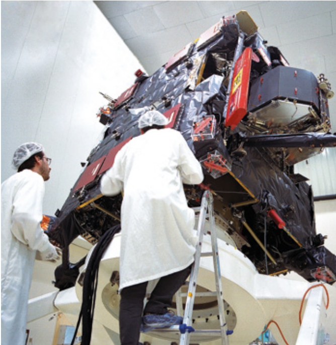
The Rosetta orbiter and Philae lander are integrated at the Guiana Space Centre before their launch by Ariane 5 on 2 March 2004 (flight 158).
